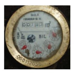
The meter reading in the above picture is therefore: 193.9037
